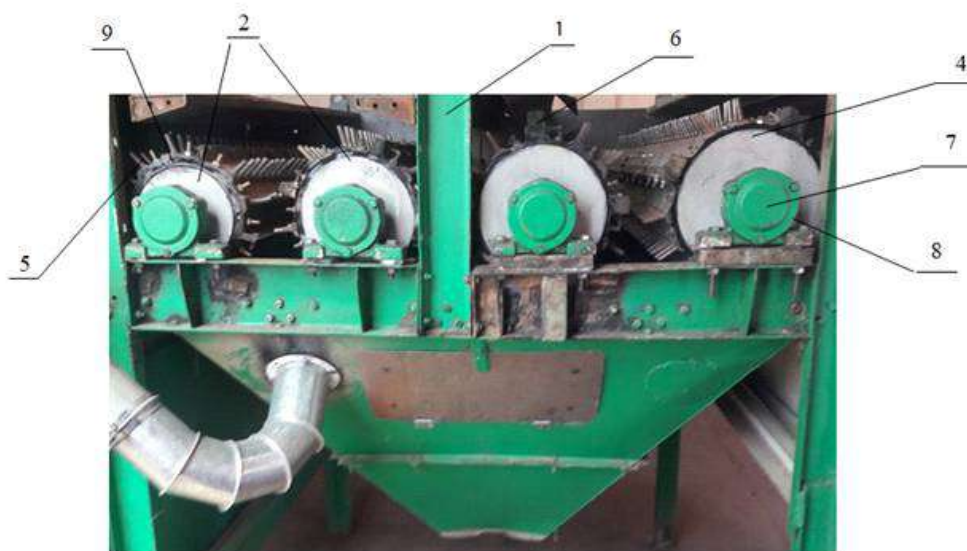
Figure 2. Cleaning section of the new improved cotton ginning unit.
