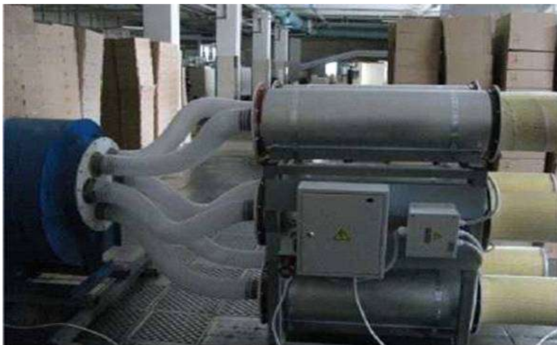
Figure 1. Equipment for disinfection of seeds in elevators or warehouses with a yield of 600 g O 3 / s of ozone-air mixture.
